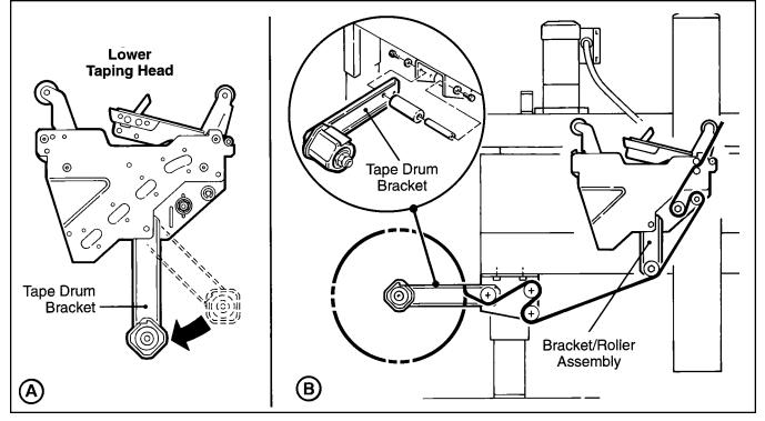
Figure 2-2 – Lower Tape Drum Bracket Position
